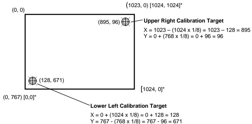
*controller's* perspective, however, place the origin at the lower left corner of the screen (numbers in brackets). The controller outputs 0 to 1024 on both axes independent of display screen resolution.
