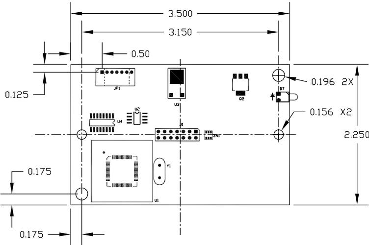
**Figure 3 Uncased EX II 17xxSC Touch Screen Controller**
