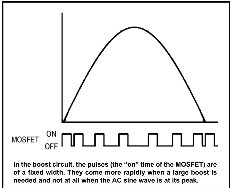
filter capacitor with narrow, harmonic-producing spikes of current, we have a steady flow of current flowing from the bridge rectifier into the filter capacitor.
