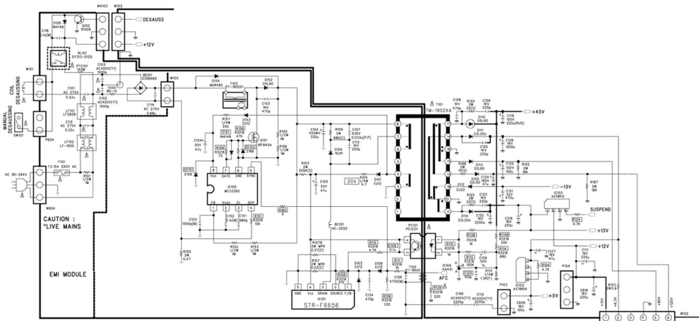
mary winding of a transformer (T103) that is turned sideways, with nothing at all connected to the secondary winding. From the right side of this transformer winding, we can follow the current path through diode D152 and then to the positive lead of our friend the filter capacitor. What is going on here? Why are there two paths and why do we have the “extra” diodes?
