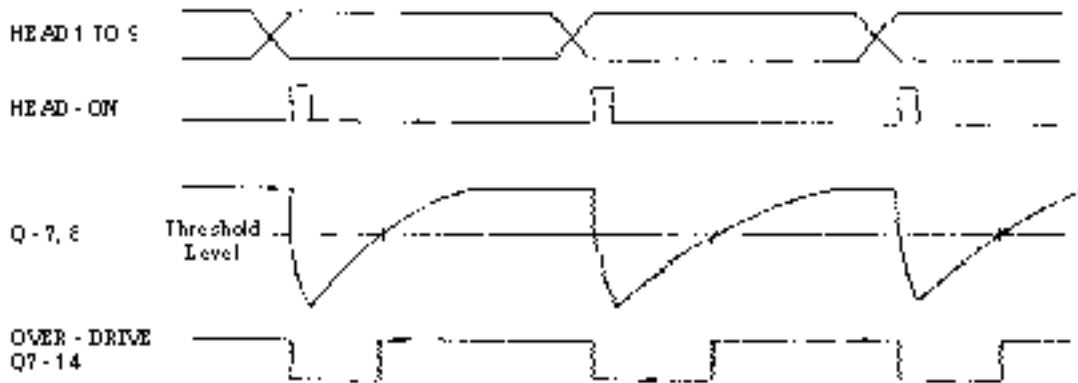
Figure 51: Communication Sequence of the Printhead Drive Circuit
