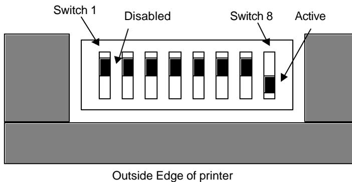
Switch 1 is the furthest to the back. The Active position is toward the outside edge of the printer.
