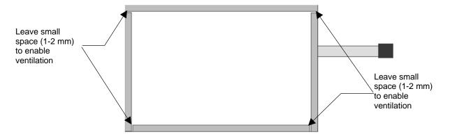
**Caution**: The tape should have a minimum thickness of 1/16 inch (1.587 mm) Avoid using thinner tapes. If thicker tape is needed, it is okay to double the recommended VHB tape. Do NOT use highly compressible tapes.
