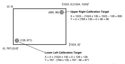
controller's perspective, however, place the origin at the lower left corner of the screen (numbers in brackets). The controller outputs 0 to 1024 on both axes independent of display screen resolution.
