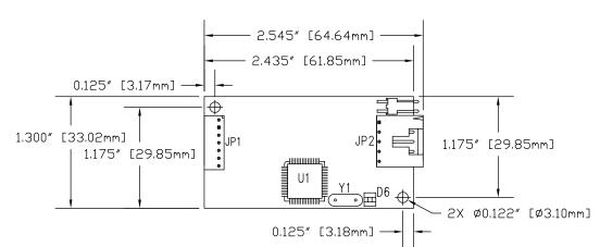
Figure 2. EX II 7720SC Overall Dimensions
