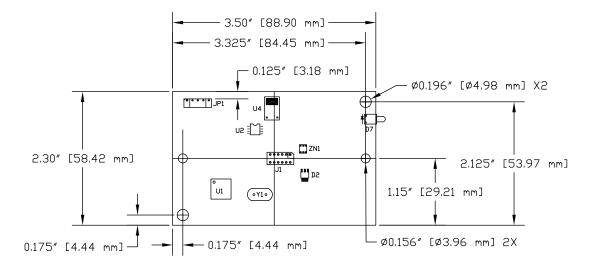
Figure 2 Cased EX II 57xxUC Touch Screen Controller
