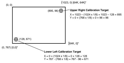
\*The coordinates are in *video* terms, with the origin (0, 0) in the upper left corner of the screen. Examples from the *controller's* perspective, however, place the origin at the lower left corner of the screen (numbers in brackets). The controller outputs 0 to 64K on both axes independent of display screen resolution.
