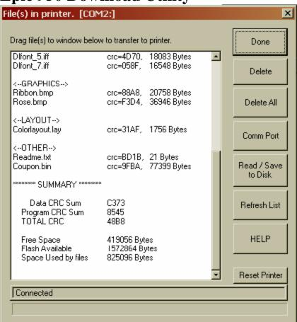
This utility allows you to query, read, and send information to your Epic 950 printer. The main display of the download utility displays printer data contents as files. This tool can be used to transfer any type of data; including graphics, ticket layouts, fonts, etc. You must load the files you export from the Ticket Layout Editor into the printer using this download utility.
